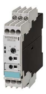
TIME RELAY, MULTI-FUNCTION 1 CHANGEOVER, 8 FUNCTIONS, 15 TIME SETTING RANGES AC/DC 24 V AND AC 200... 240 V WITH LED, SCREW CONNECTION
